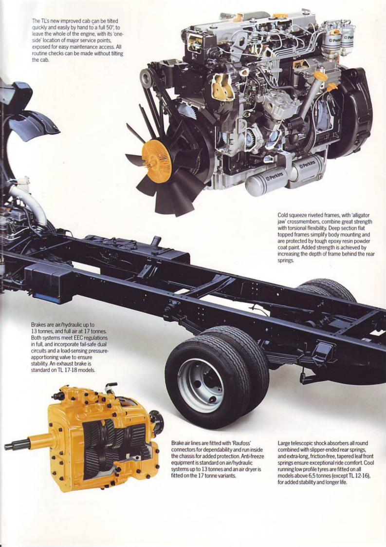
The highly acclaimed Perkins Phaser engines create new standards in power, economy and reliable long life, providing TL users with high productivity and low operating costs. The 6,0 litre turbocharged engines offer excellent low end torque and high torque rise over a broad operating range for good startability and unrivalled flexibility in traffic or on steep grades.
