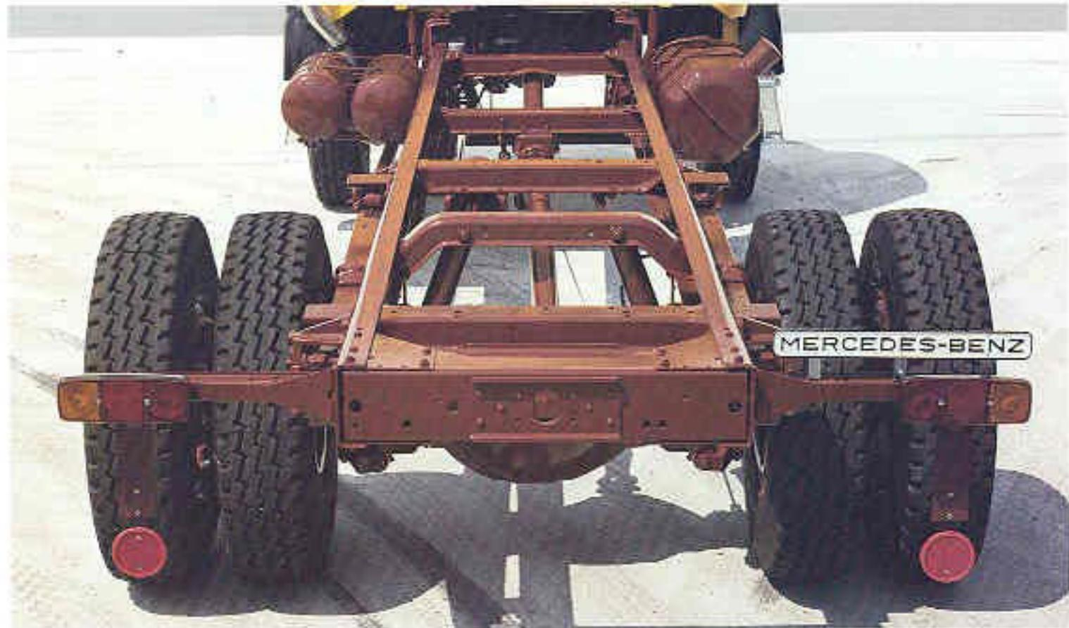
The frames for dropside and dump trucks are made of sturdy U-section longitudinal members to which cross-members are riveted to give high torsional flexibility. The front cross-member takes the coupling jaw and pin. The rear cross-member can be fitted with a trailer coupling. Engine and gearbox are suspended on rubber vibration dampers. The special double frame of the semitrailer tractors is reinforced by L-shaped longitudinal members. This considerably improves torsional resistance.
