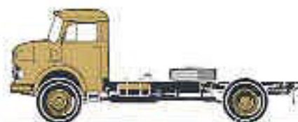
LA 911 B, all-wheel drive chassis Wheelbase 165.3 in. (4,200 mm) Payload and body allowance 12,200 lbs. (5,535 kg)
