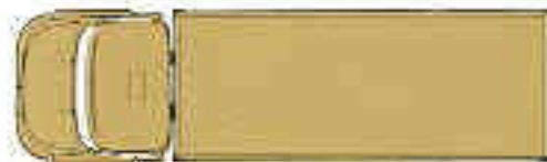
L 911 B Wheelbase 190.2 in. (4,830 mm) Payload and body allowance 12,885 lbs. (5,845 kg) Recommended body size 208.7 x 92.5 x 19.7 in. (5,300 x 2,350 x 500 mm)
