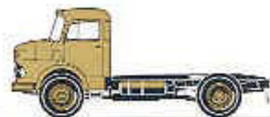
LS 911 B, tractive unit Wheelbase 141.7 in. (3,600 mm) Fifth wheel load 12,950 lbs. (5,875 kg) Perm. gross combination weight 40,300 lbs. (18,300 kg)
