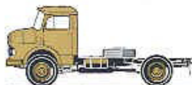
LA 911 B, all-wheel drive chassis Wheelbase 141.7 in. (3,600 mm) Payload and body allowance 12,270 lbs. (5,565 kg)
