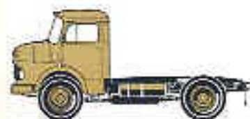
LS 911 B, tractive unit Wheelbase 128.0 in. (3,250 mm) Fifth wheel load 13,050 lbs. (5,930 kg) Perm. gross combination weight 40,300 lbs. (18,300 kg)
