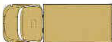
L 911 B Wheelbase 141.7 in. (3,600 mm) Payload and body allowance 13,085 lbs. (5,935 kg) Recommended body size 141.7 x 98.5 x 19.7 in. (3,600 x 2,500 x 500 mm)
