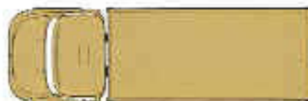
L 911 B Wheelbase 165.3 in. (4,200 mm) Payload and body allowance 12,965 lbs. (5,885 kg) Recommended body size 177.2 x 92.5 x 19.7 in. (4,500 x 2,350 x 500 mm)
