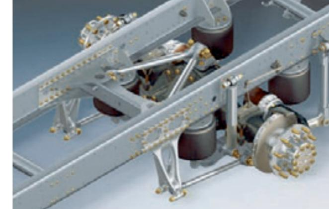
4-bellows rear-axle air suspension for the TGM.
