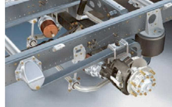
2-bellows rear-axle air suspension for the TGL.
