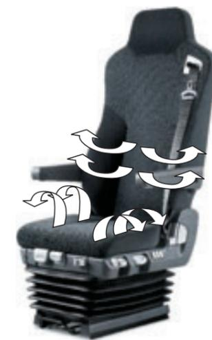
Air-sprung driver's comfort seat with integrated belt system and optional armrests.
