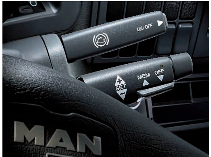
Steering Column Stalk. (MAN TipMatic)
