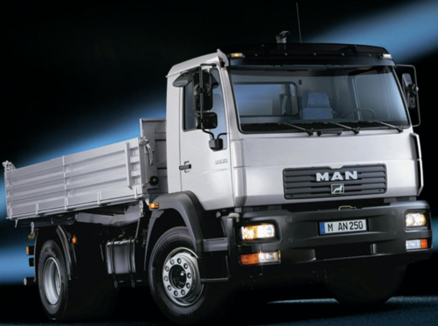
**THE IDEAL FRAMEWORK.** Level from back to front, the ladder-type frame is a role model in body-friendliness and stable – no components jut out over the upper edge. It has optimised weight and is highly robust thanks to tubular cross members, which protects the body whilst ensuring excellent ride stability. For safety, the series M2000 Evolution is fitted with underride protection at the rear as well as on the sides, if necessary. A similar device at the front is available as an optional extra.
