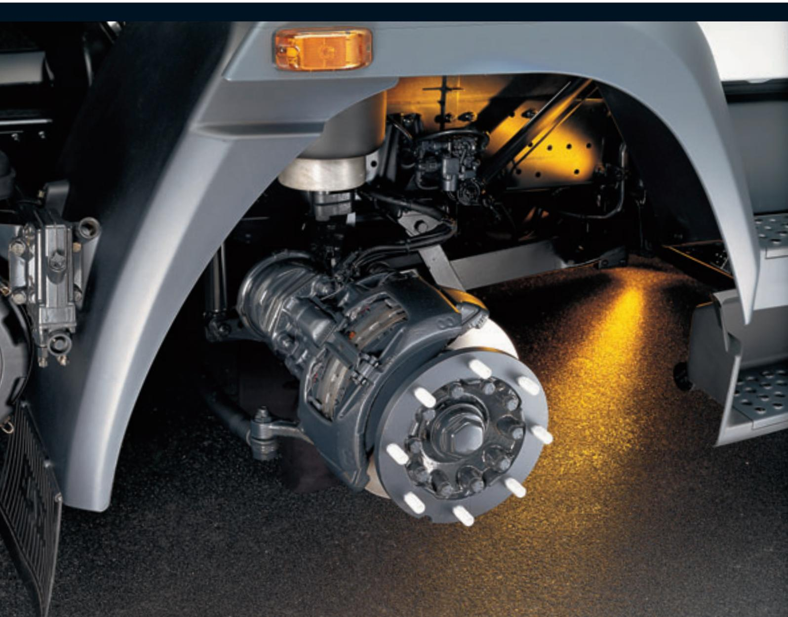
**RIDE SAFELY, BRAKE SAFELY.** When it comes to braking distance, the M2000 Evolution's motto is "a little is more." That's why it has air-actuated and internally ventilated disk brakes on the front axles. Low-abrasive s-cam and/or wedge drum brakes with automatic brake shoe readjustment make for reliable performance at the rear. On all-wheel drive versions, drum brakes are used on every axle.
