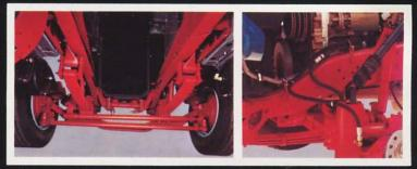
With Mack's axle-mounted steering gear and steering geometry, wheel kick is virtually eliminated, even under the most severe road conditions. You get optimum road feel with minimum steering effort for a safer, less fatiguing ride. Entire front suspension is engineered with a 50,000-mile (80 450 km) highway service interval.
