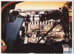
Mack's Frontal Air Intake System reduces fuel consumption and extends service life. Unaffected by sleet or snow, it is a quiet, efficient performer that features a 150,000-mile (241 350 km) service interval for its filter element when used in normal highway service.
