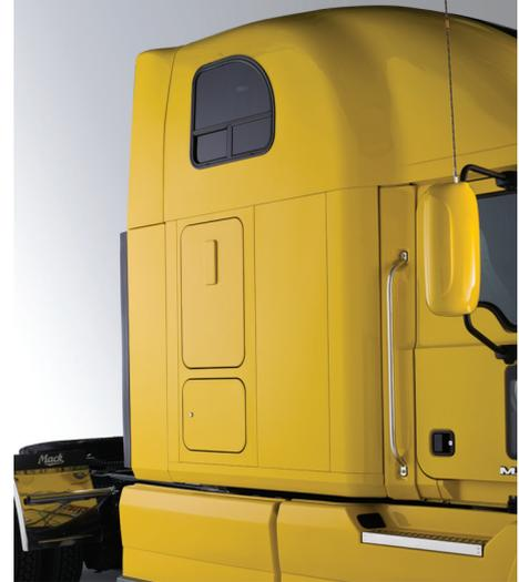
On the outside, the smooth lines of the exterior guide airflow over and around the sleeper, thanks to the full-roof fairings and side extenders that help improve fuel economy by as much as 15 percent.
