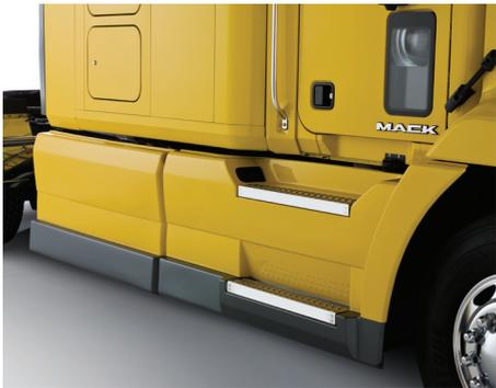
Fuel-tank fairings work with the bumper to keep air flowing smoothly along the length of the tractor. The bumper and chassis fairings also boost fuel economy.
