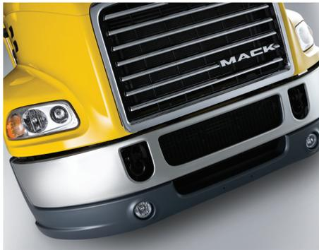
Mack's aerodynamically-designed front bumper doesn't just look good, it also moves air smoothly around and under the front of the truck.
