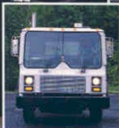
The low cab forward configuration and light wheel cuts make the MR model more agile than conventional trucks.
