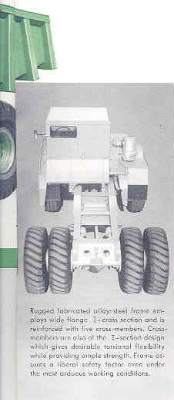
Rugged, fabricated alloy-steel frame employs wide flange I-cross section and is reinforced with five cross-members. Cross-members are also of the I-section design which gives desirable torsional flexibility while providing ample strength. Frame affords a liberal safety factor even under the most arduous working conditions.
