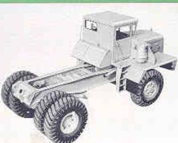
Simplified maintenance of air cleaner is afforded by readily accessible mounting on right hand side of cab. Unit is fully protected by cab canopy.
