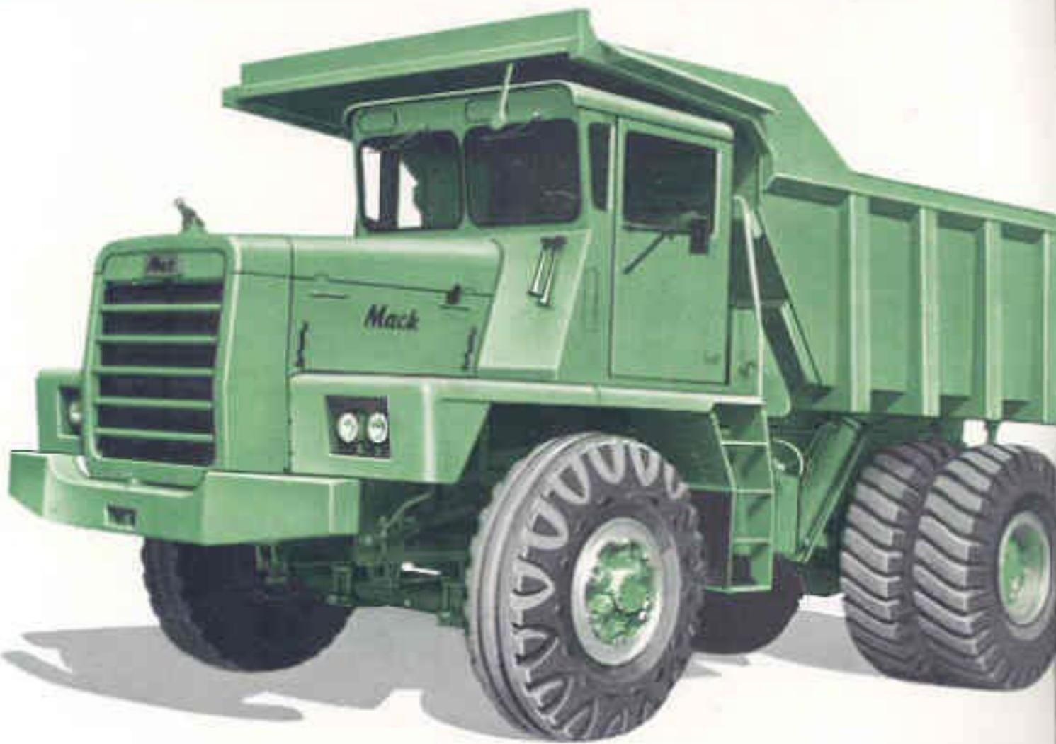
Driver comfort is assured by convenient arrangement of controls and instruments, as well as adequate ventilation in this roomy cab offset to the left, thereby providing excellent vision both fore and aft and to the sides.
