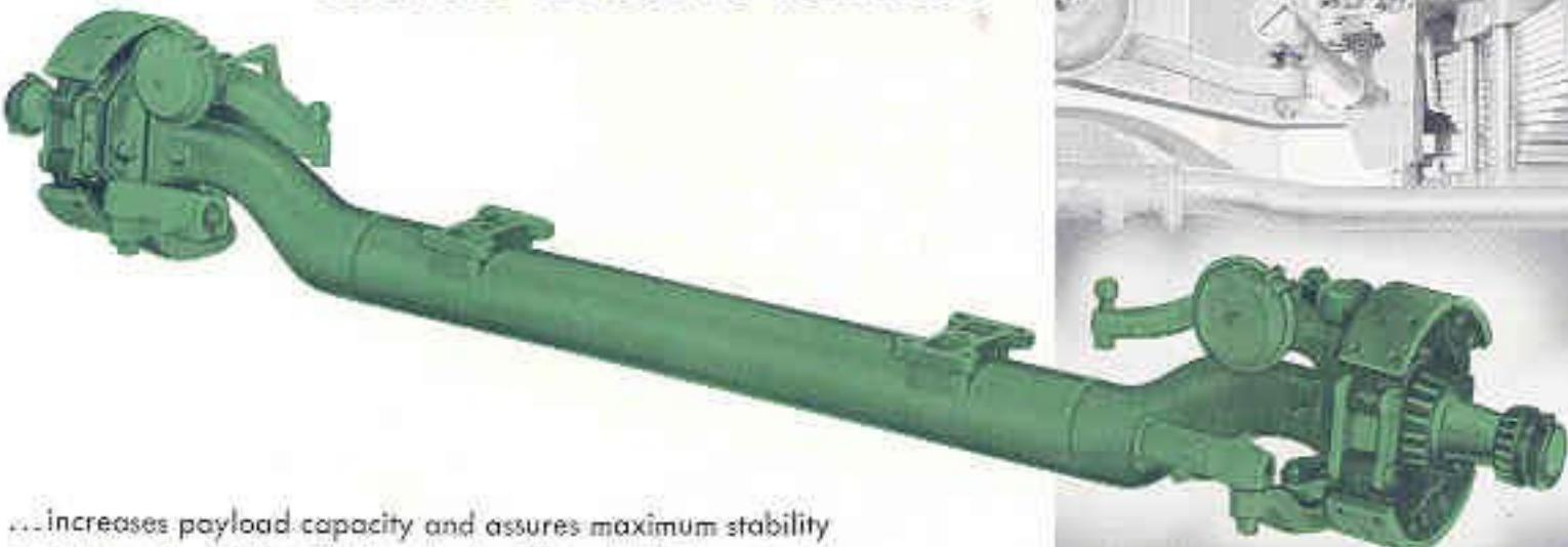
...increases payload capacity and assures maximum stability and strength with its 7" diameter by  $\frac{3}{4}$ " wall thickness tubular construction and tread of 107". Weighing more than 2300 lbs., the reversed-elliot FA-900 Mack front axle will withstand the most rugged extra-heavy duty service.
