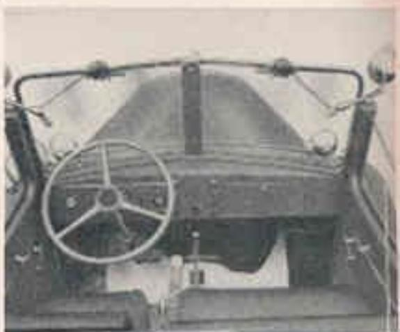
Comfort of accommodations and convenience of operating controls receive special attention in Mack design. Note individual, adjustable driver's seat and handy, out-of-the-way location of parking brake.
