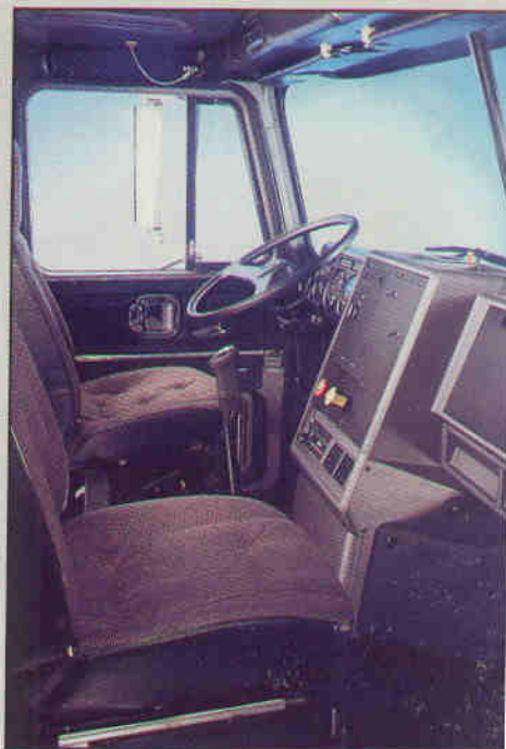
CH600 Preferred Series interior in silver gray. Features such as a back wall storage compartment and overhead lighting console add convenience. Multi-speed transmissions are controlled with a new, ergonomically designed multi-function air shift lever, and a removable floor hatch surrounding its base provides easy transmission access.
