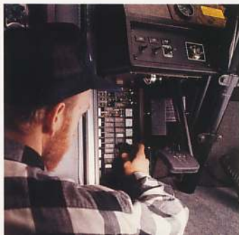
The power distribution box puts all circuit protection elements in one central, lighted location that's close at hand.
