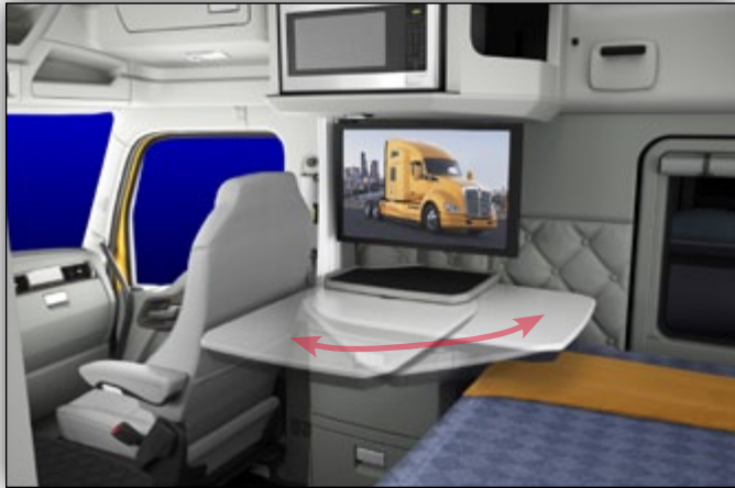
Sturdy work/ dining table swivels for easy access from bunk or passenger seat (which rotates 180 degrees).
