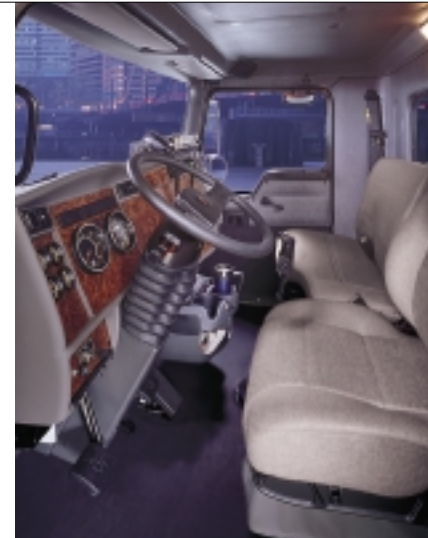
A cut above other trucks in its class, the T300 sports a great looking, well-ventilated, fully-trimmed, quiet and spacious interior – part of Kenworth's strategy to help you attract and retain quality drivers. In-cab storage features include an oversized glove box and a tool box located under the rider's seat offering an additional three cubic feet of space.
