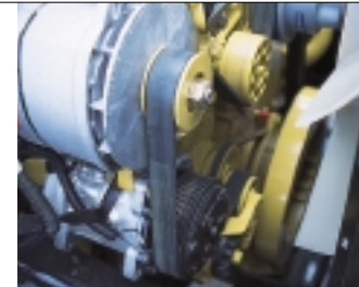
A single poly "V" belt drives all engine accessories, which means fewer parts to stock, of course. But the best part? It can be replaced in less than 10 minutes with no special tools.
