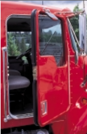
Thick, insulated bulkhead-type doors swing true and easy on continuous piano hinges made of stainless steel for long life.
