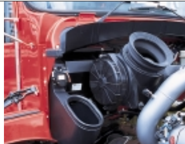
The heater/air conditioner motor – a pain to find and uncover in most trucks – is also mounted on the firewall for faster replacement or repair.
