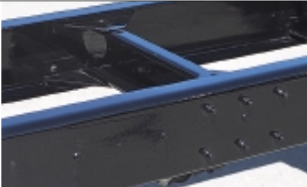
Kenworth's frame is a continuous straight steel rail custom-drilled to specification. Steel cross-members and gussets for added strength are Huck bolted to ensure you have the additional foundation you need to meet the daily demands you will place on the T300. The result: a trouble-free frame of unsurpassed integrity and strength.
