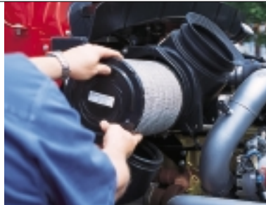
Changing an air filter is straightforward, quick and easy to do.
