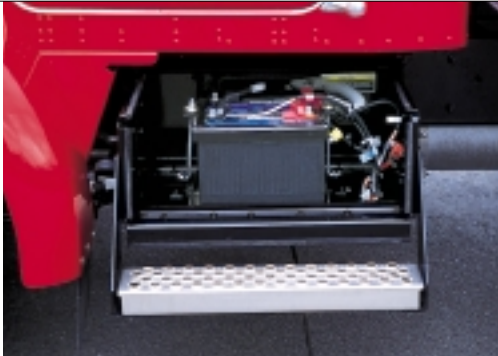
Here is another reason Kenworths are so dependable: 12-volt maintenance-free batteries placed in a corrosion-resistant, shock-absorbing rubber tray, held firmly in place and mounted on the left-hand side, close to the starter motor for minimum voltage drop.
