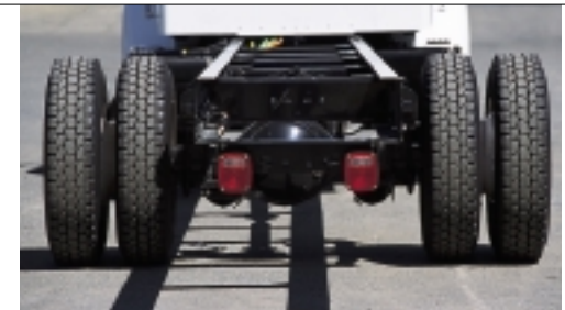
The T300's frame offers a clean top flange from back-of-cab to end-of-frame. Nothing to get in the way of an efficient body installation.
