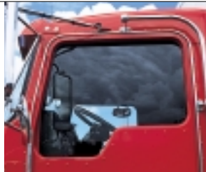
Kenworth's innovative Daylite® doors increase visibility and reduce the "blind spot" – especially critical on busy and often constricted city streets.
