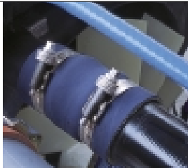
A standard item on Kenworth trucks, constant torque hose clamps go on tight and stay that way.
