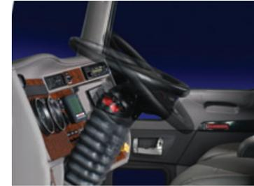
*Tilt and telescoping steering column.*
