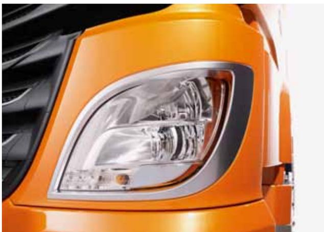
**INNOVATIVE** A first in the truck industry is the optional LED technology for the headlights. With the largest light output, maximum life and minimal energy consumption. Standard daytime running lights provide excellent daytime visibility. Cornering lights (optional) in the bumper shine in the driving direction for extra safety and less risk of damage. Bulbs can be replaced quickly thanks to practical inspection hatches.
