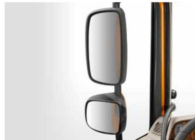
**VISIBLE** The door window offers the driver maximum side visibility. The driver can see both between the mirrors and A-pillar of the cab, and even between the mirrors themselves. This gives good visibility for maximum safety.
