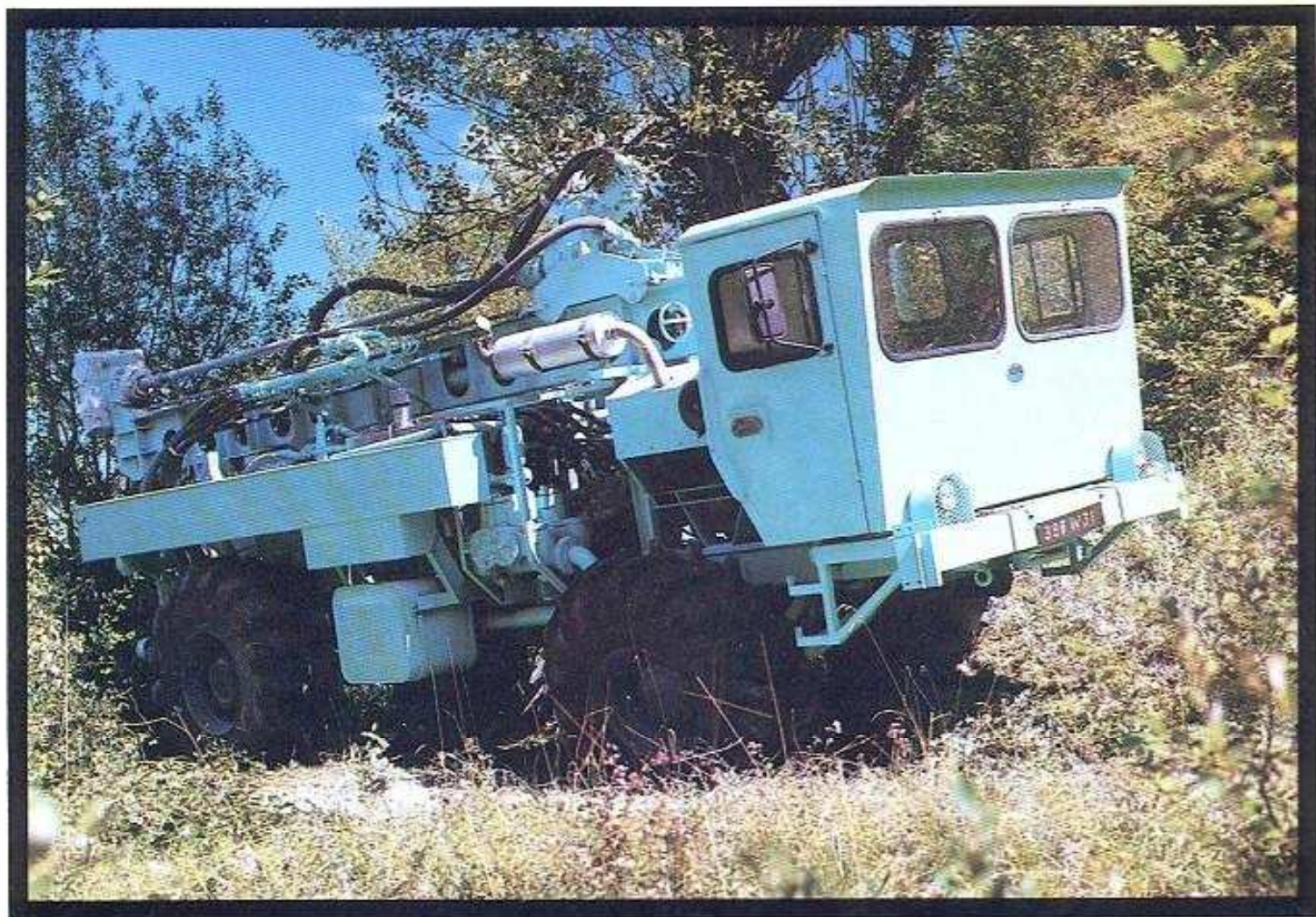
VATT P 14 MOUNTED AS DRILL RIG CARRIER
