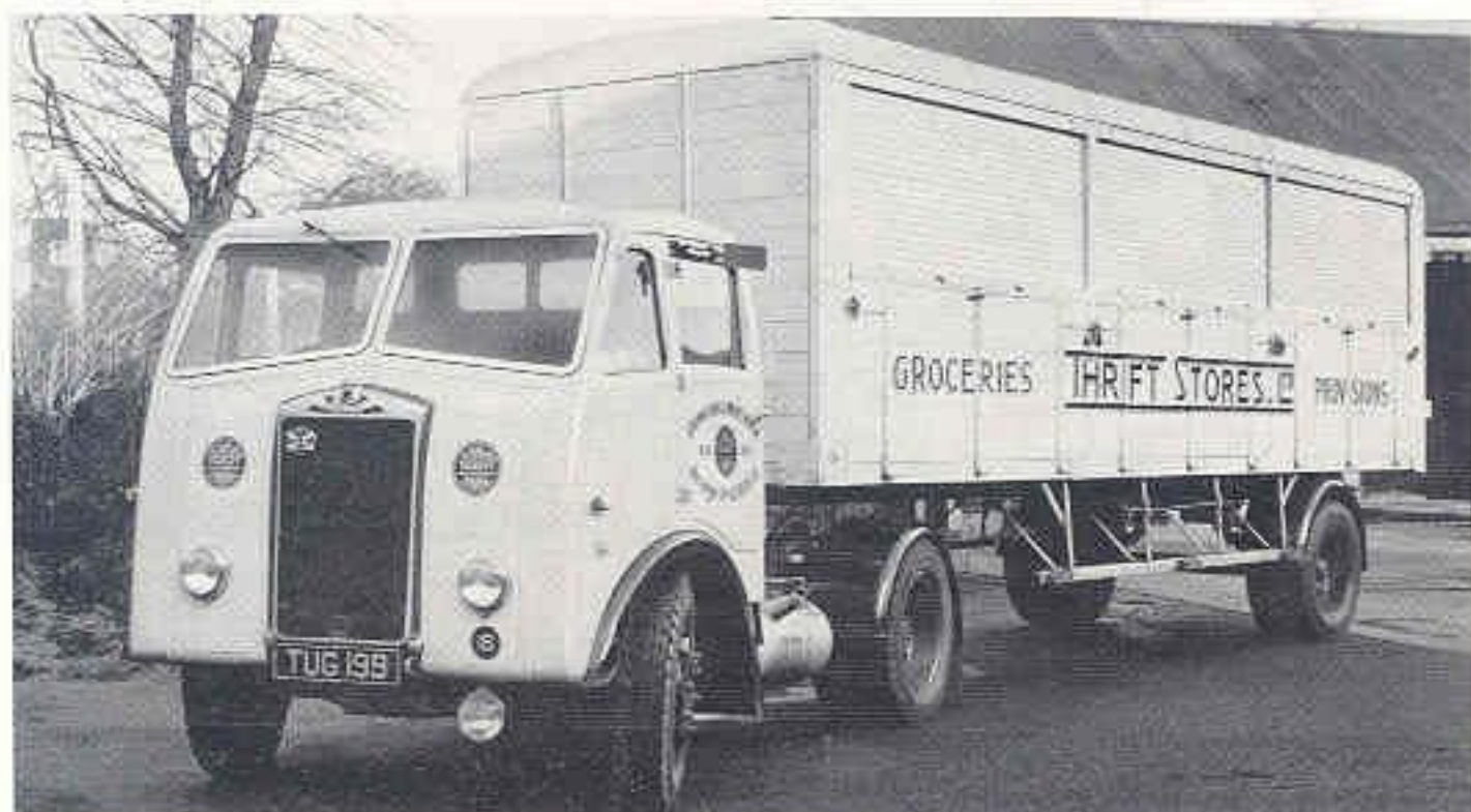
ALBION-SCAMMELL Tractor with anti-trailer van - capacity 1000 cu. ft.
