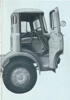
The cab is of entirely modern design with every feature essential to the vehicle of today. Particular emphasis has been placed on ease of entrance, visibility and driver comfort. It is a pressed-steel welded assembly based on a rigid sub-frame of deep box section pressings, combining strength and durability with pleasing lines and styling.
