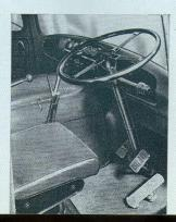
Readily accessible controls, which include organ pedal accelerator, cut driving effort to a minimum, thus reducing fatigue on long distance journeys. Instruments are grouped in an attractive detachable panel with concealed illumination, and mounted in easy-viewing position. Floor of cab has rubber mats and pedals and doors are draught sealed.
