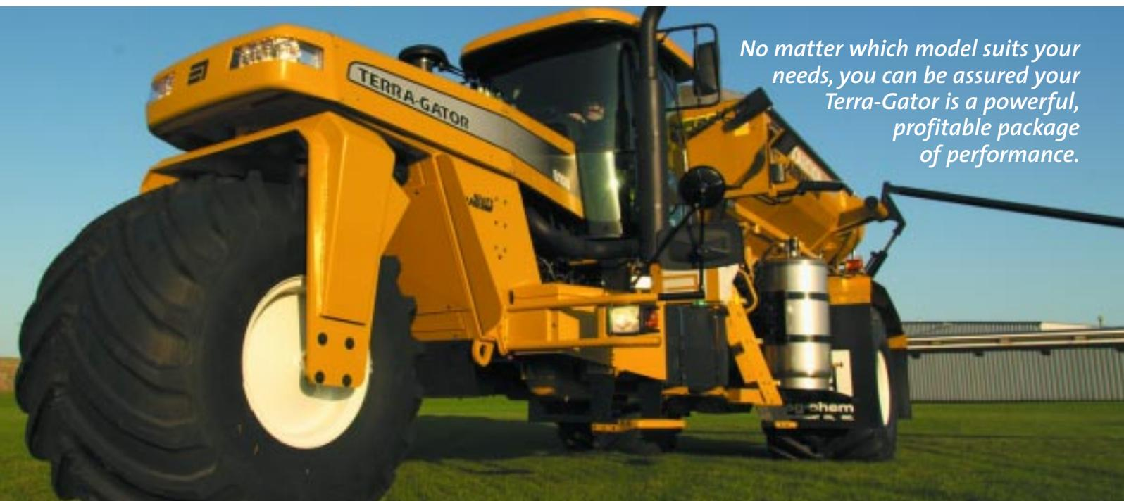
Keep your costs down and your productivity up. The Terra-Gator 6103 is a rugged machine designed exclusively for use with an 1,800-gallon liquid or spinner spreader. The 130-gallon fuel capacity lets you run a long day without refueling.
