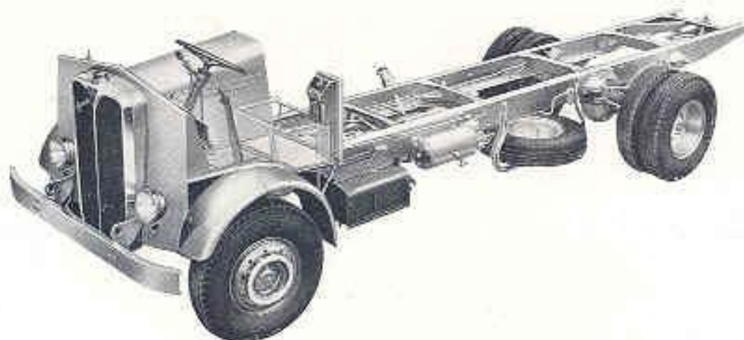
ARRANGEMENT OF THE 14 ft. 7 in. WHEELBASE CHASSIS
