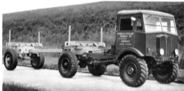
For heavy transport of loads under the most arduous conditions, the 4-wheel drive "Matador" is unrivalled. This machine, working with a crawler trailer, operates on the roads and in the forests of the Gold Coast.
